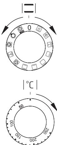
The oven can be switched off by setting both of these knobs to the position “●”/“0”.
