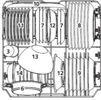
Tests specification according to EN 60436
