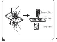
3. Larger residues can be rinsed under running water. Clean the filter completely with a soft, clean brush.
