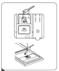
Add detergent into the larger cavity (A) for the main wash cycle. For better cleaning result, especially if you have very dirt items, pour a small amount of detergent onto the door. The additional detergent will activate during the pre-wash phase.
