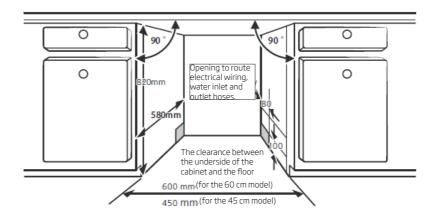
2. When installing the dishwasher in the corner cupboard, leave room for the door to open.
