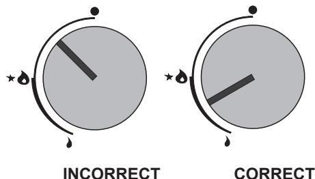
This example shows you how to operate the knob and adjust flame size.
