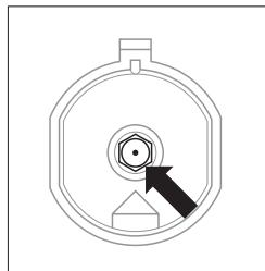
Replace burner nozzle: unscrew the nozzle using a special wrench no. 7 and replace with a new one suitable for the new gas type (see table above).
