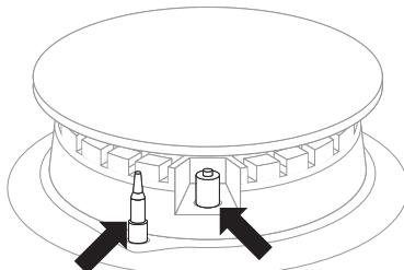
In hobs equipped with a flame-failure cut-off device, hold the pushed down knob in the "large flame" position for approximately 10 seconds to activate the a flame-failure device
