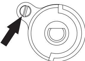
In order to check the flame, heat up the burner on a full flame for about 10 min., and then turn the burner knob to an economic flame position. The flame should not go out or jump on the nozzle. However, if it does, readjust of the valves.
