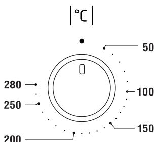
The oven can be switched off by setting both of these knobs to the position “●”/“0”.
