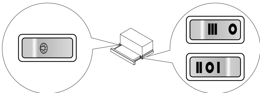
The control panel is equipped with buttons (rocker switch). You can use the buttons once the retractable front panel is ejected.
