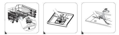
1. To remove the upper spray arm, hold the nut in the center still and rotate the spray arm counterclockwise to remove it.
