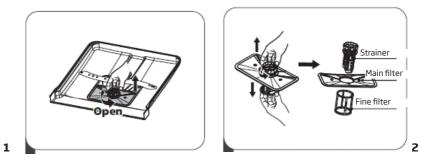
1. Hold the strainer and turn it counter clockwise to unscrew. Lift the filter up and remove it from the dishwasher.
