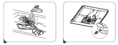
3. Larger residues can be rinsed under running water. Clean the filter completely with a soft, clean brush.
