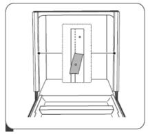
Remove the protection from the sound-absorbing strips, then stick the strips to the side plates, please align to the hole postion.
