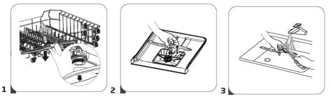
1. To remove the upper spray arm, hold the nut in place and turn the arm counter clockwise.
