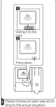
1. Open the cap by sliding the release catch.
