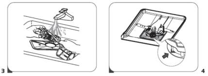
3. Larger residues can be rinsed under running water. Clean the filter completely with a soft, clean brush.
