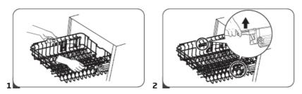
1. To raise the basket to the upper position, raise it until it is at the same height on both sides. Make sure it is securely attached to the rails.
