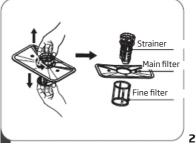
1. Hold the strainer and turn it counter clockwise to unscrew. Lift the filter up and remove it from the dishwasher.
